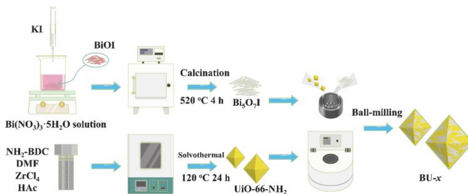
Fig. 1. The fabrication procedure of the BU-x heterojunctions.
